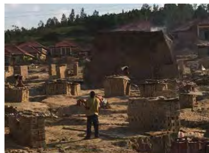
Traditional brick burning with fuel wood
